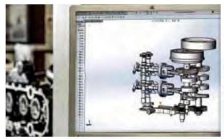
All of the moving parts of the vertically-mounted Dtorque engine are clearly seen in this CADCAM screen display. Central to the assembly are the dual crankshafts with their miniature counterrotating flywheels. Light weight connecting rods are connected to crankshafts by two inline pistons, while aspiration is provided by four camshaft-driven valves per cylinder.
