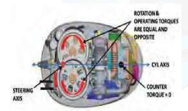
This two-dimensional diagram shows clearly how the two reciprocating pistons complement each other at the full extent of their up and down strokes. It may look simple, but the asymmetric engine cycle with its short compression stroke, longer intake stroke and shorter expansion stroke required particular attention from the NEANDER Dtorque engineering design team. The benefit, however, is improved thermal efficiency with an extended piston work stroke.
